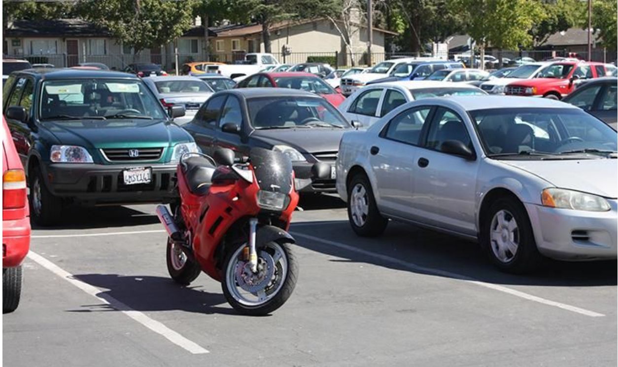
Figure 14. Smaller vehicles may not show up on the rangefinder distance readings if they are parked on one side of a space or the other. Image: The American River Current.
