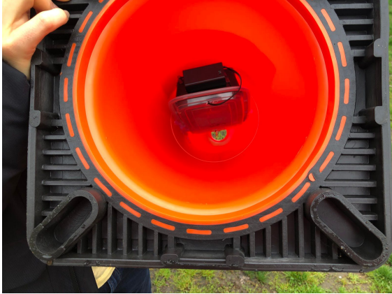
Figure 5. Arduino is held with double-stick tape inside a plastic container, with wires connecting to the sensor. This setup is short-term weatherproof and would need significant upgrades for long-term use. As a prototype, it was completely functional and would be reconfigured with considerations when developed at scale.
