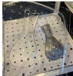
Vacuum forming tool used to thermo-mold tasset replica
