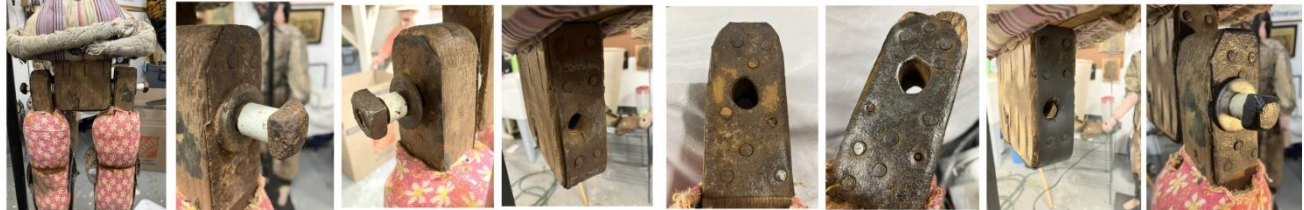
Pelvis and leg joint hardware showing rust and corrosion, removal and treatment with neutralizer/sealer.
