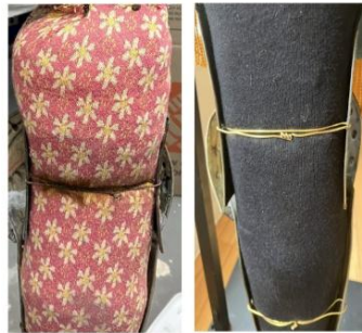
Rusted and soft brass wire
